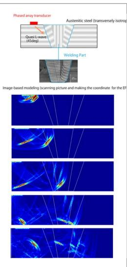
Ultrasonic wave propagation in the anisotropicsteel with a welded part. The crystalline orientations of welding part are different from austenitic material steel.
