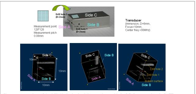
Shape reconstructions of the drilled holes in aluminium specimen with the 3-D frequency domain SAFT.
