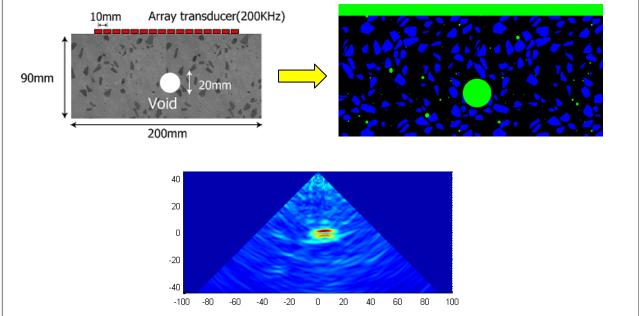
Image based EFIT modeling of concrete material (upper figure) and imaging of void by the time domain SAFT-combined with revolutionary filtering techniques (bottom figure).
