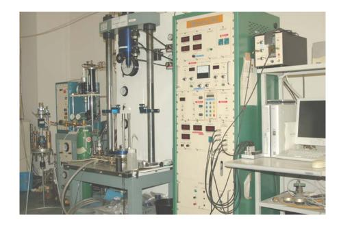
Cyclic triaxial apparatus is used to investigate soil behavior under cyclic loading. The apparatus in Ehime University has special equipment so that not only pore water pressure but pore air pressure is independently controlled during tests.
