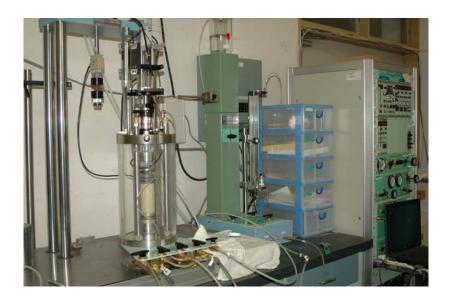
Ehime University Cyclic triaxial apparatus with servo controlled pneumatic cylinder can precisely control stress state of specimens. This is mainly used to perform liquefaction tests on soils used for centrifuge models and on materials obtained from in-situ. High-quality undisturbed samples obtained by grand freezing method are sometimes tested in this apparatus.
