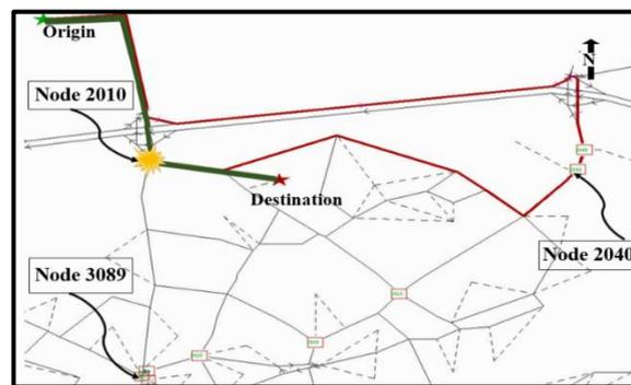
Fig.4. Optimum path obtained from SATURN without a blockage (green) and with a blockage (red)
