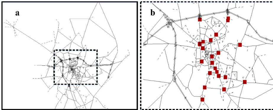
Fig. 3. (a) Cambridge network modelled in SATURN; (b) The 24 signalized intersections represented by red squares
