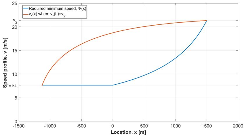
Fig. 4: Numerical calculation of speed profile under optimal conditions.
