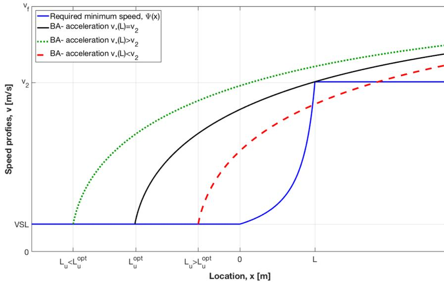
Fig. 2: Illustration on required speed at each location. The dashed-red speed profile is unfeasible, while dotted-green is feasible but not optimal. Only when  $v_*(L) = v_2$  the control was implemented at the optimal application area, i.e. black speed profile.
