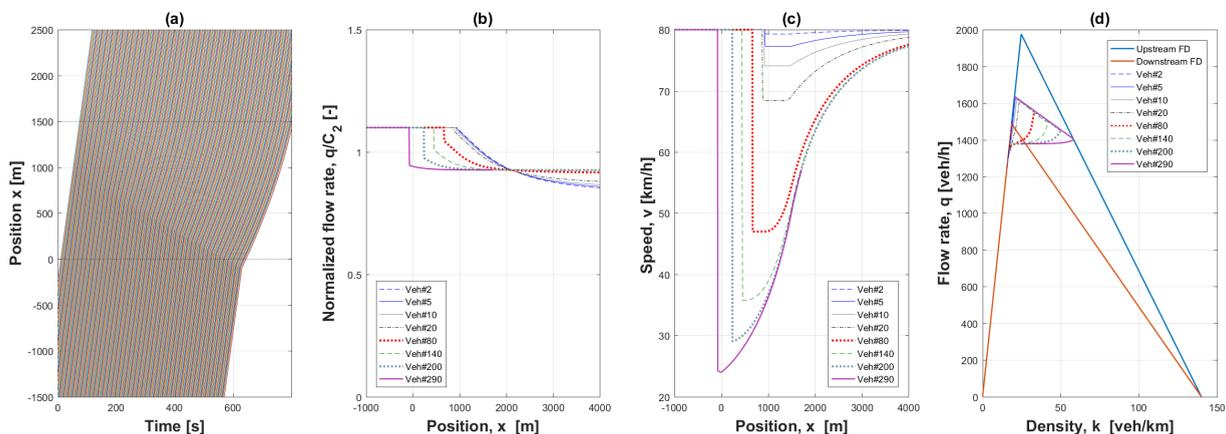
Fig. 3: (a) Trajectories of 300 vehicles. (b) Normalized flow rate (over downstream capacity) for several vehicles. (c) Speed profile of different vehicles. (d) Temporal evolution of traffic states for different vehicles.
