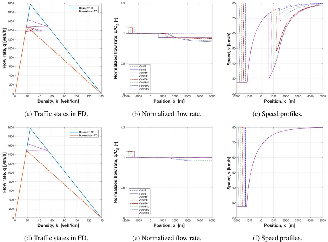
Fig. 5: (a)-(c) Control at  $L_u = -1140$ . After several vehicles break down the acceleration process inside the bottleneck is defined by LWR states and not bounded by the BA model. Capacity drop appears. (d)-(f) Control at  $L_u = -1170$ . Stationary speed profiles, acceleration of vehicles is bounded by BA model at all locations. Capacity drop prevention.
