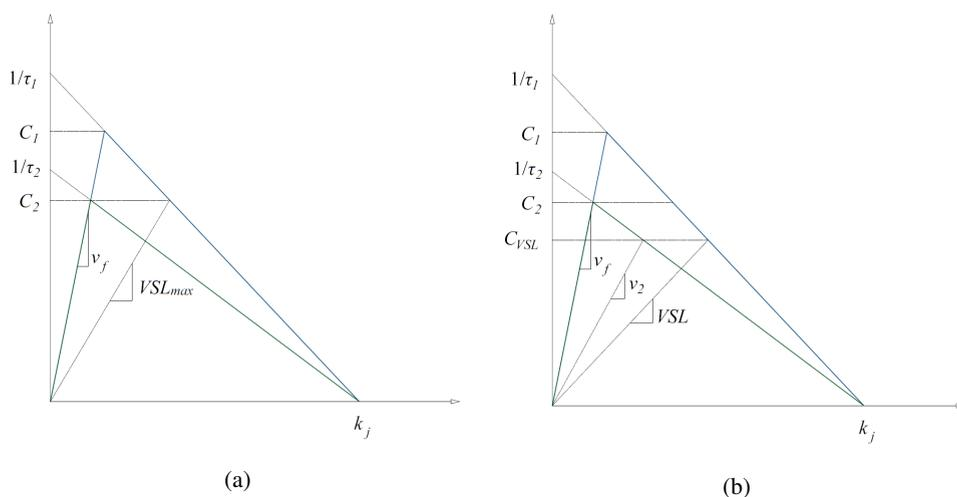
Fig. 1: (a) Maximum speed limit,  $VSL_{max}$ , defined by downstream capacity,  $C_2$ . (b) Lower speed limit and its associated flow rate,  $C_{VSL}$ , and speed for congested downstream states,  $v_2$ .
